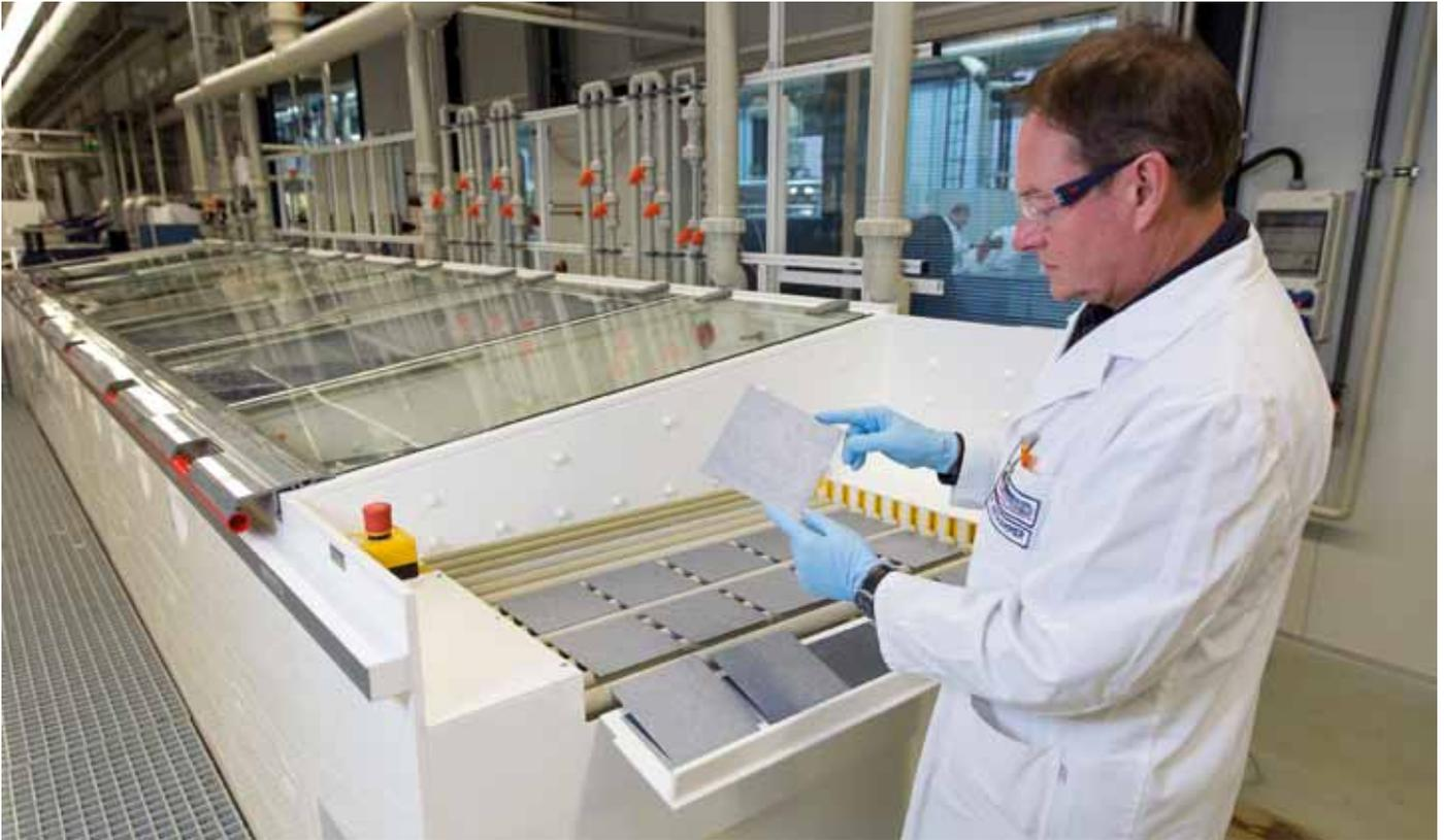
Germany's Schmid has developed the DW PreTex solution to allow manufacturers to adopt diamond wire sawing for multicrystalline silicon.
